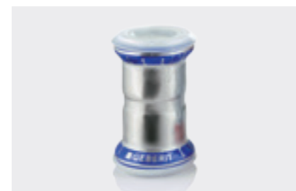
↑ GEBERIT MAPRESS STAINLESS STEEL: PRODUCT MATERIAL 1.4401 Checked and approved for dry and wet sprinkler systems by VdS and FM Approvals (among others) and suitable for use in dry and wet extinguishing water pipes in accordance with DIN 14462.
