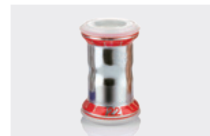
↑ GEBERIT MAPRESS CARBON STEEL: PRODUCT MATERIAL 1.0034, 10215 Checked and approved for wet sprinkler systems by VdS and FM Approvals (among others) and suitable for use in wet extinguishing water pipes in accordance with DIN 14462.
