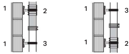
Figure 63: Transition with Geberit clamp, Geberit HDPE always with support ring
